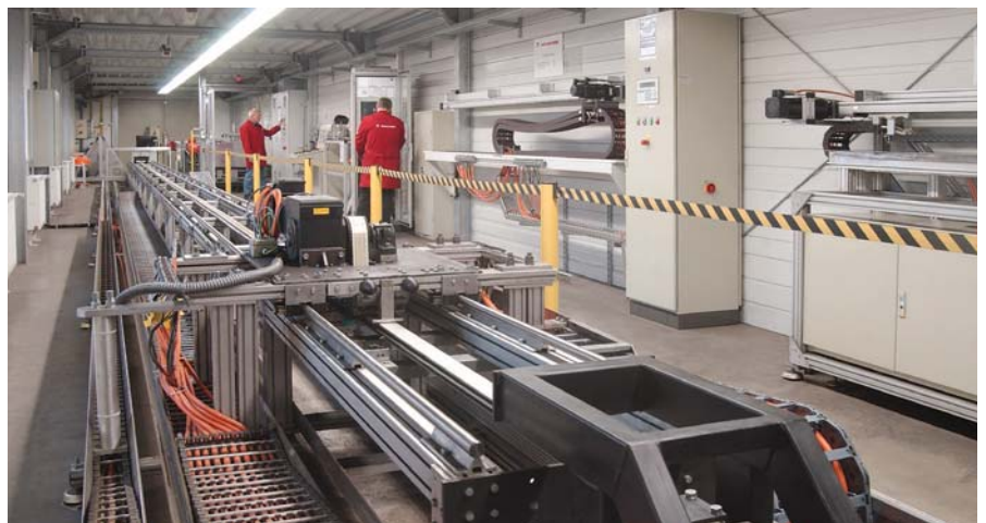
Drag chain test system
